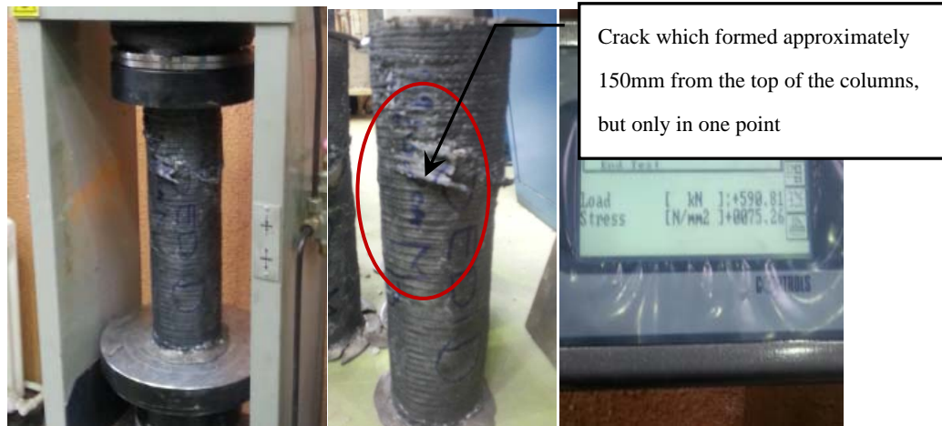
Fig.2. Test set up and shape of failure of circular specimens
