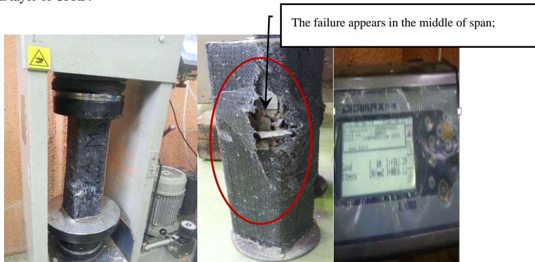
Fig.3. Test set up and shape of failure of rectangular (fully wrapped) specimens
